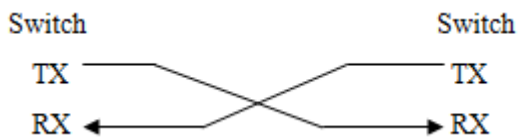
Figure 7-4 Fiber-Optic Cable Connection
