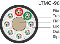
Fibre Tube filling compound FRP strength member Loose tube Outher sheat Ripcord
