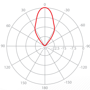
V/H - Port Pattern Elevation 5.6 GHz
