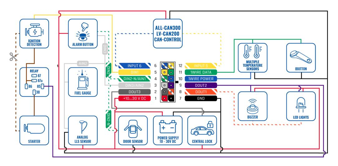
Figure 3 FMM130 Wiring scheme
