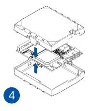
Figure 7 Attaching cover back
