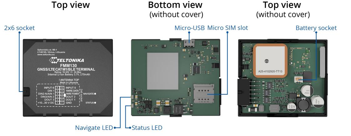
Figure 1 FMM130 device view
