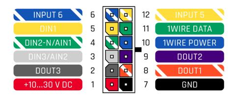
Figure 2 FMM130 2x6 socket pinout
