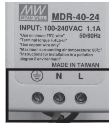
**Figure 1.** Connect the 3 lines from AC Power Cord Cable to the corresponding location.
