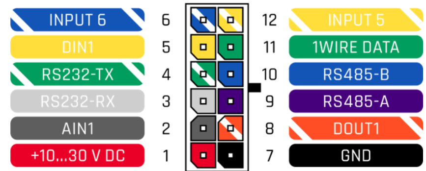
Figure 2 FMM125 2x6 socket pinout
