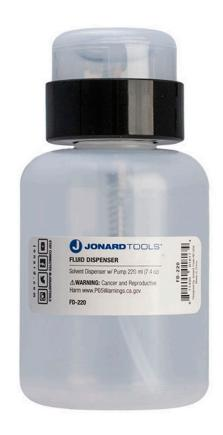
The FD-220 Fluid Dispenser is designed to store and dispense cleaning fluids, such as isopropyl alcohol, to clean the end-faces of fiber optic cables. With a spill-proof lid, 220 ml capacity, and suction pump, this fluid dispenser is the most convenient way of carrying and dispensing cleaning fluid.
