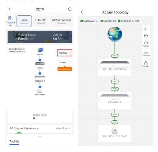
(2) Tap the **Topology** button, and select the existing managed device. To add an unmanaged downlink switch manually, select **Manually Add**.
