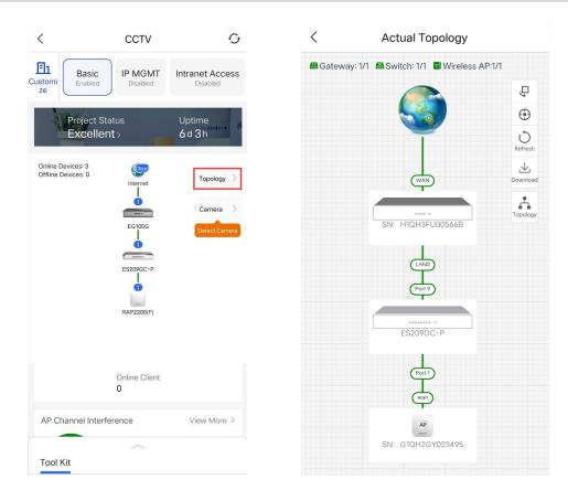
(2) Tap the **Topology** button, and select the existing managed device. To add an unmanaged downlink switch by scanning its QR-code, select **Scan to Add**.
