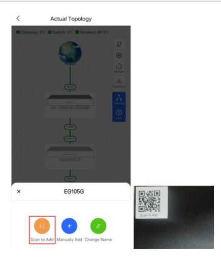
(3) After the device is detected, select its uplink port. And the device is added successfully.
