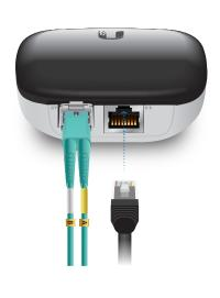
Connect an Ethernet cable from a device delivering PoE to the UF-AE.
