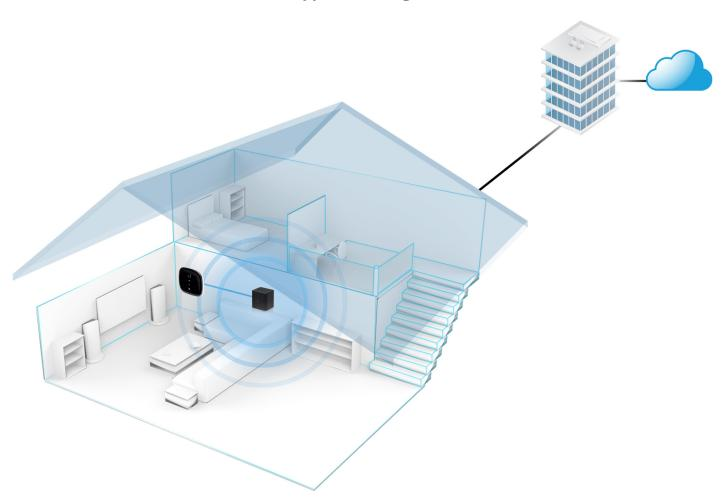
The UFiber Active Ethernet delivers active fiber from the service provider to the customer's residence, where it is powered by the airCube™ AC, model ACB-AC.
