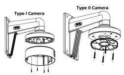
Figure 2-11 Attach the Back Box/Base Plate to the Bracket
