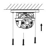
Figure 2-7 Fix the Mounting Base
