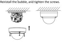
Figure 2-9 Bubble Reinstallation
