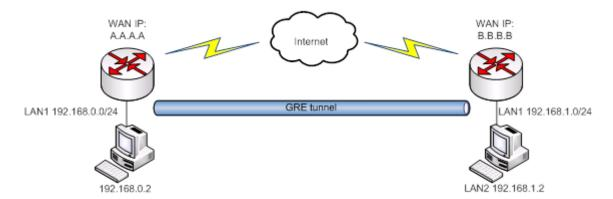
In the example network diagram two distant networks LAN1 and LAN2 are connected.
