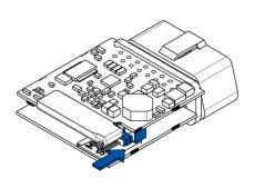
Figure 5 Battery connection
