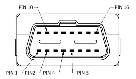
Figure 2 FMB010 OBDII socket pinout
