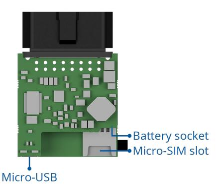
Figure 1 FMB010 device view
