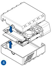
Figure 6 Attaching cover back
