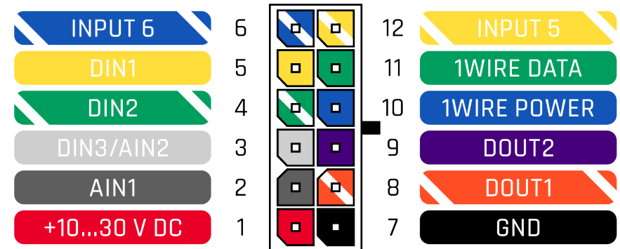
Figure 2 FMB110 2x6 socket pinout
