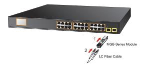
Figure 3-4: Plug In the SFP Transceiver
