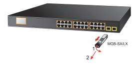
Figure 3-5: How to Pull Out the SFP Transceiver
