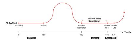
Figure 2-4: Alive Check Mechanism
