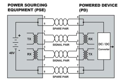
Figure 1: Power Supplied over Spare Pins
