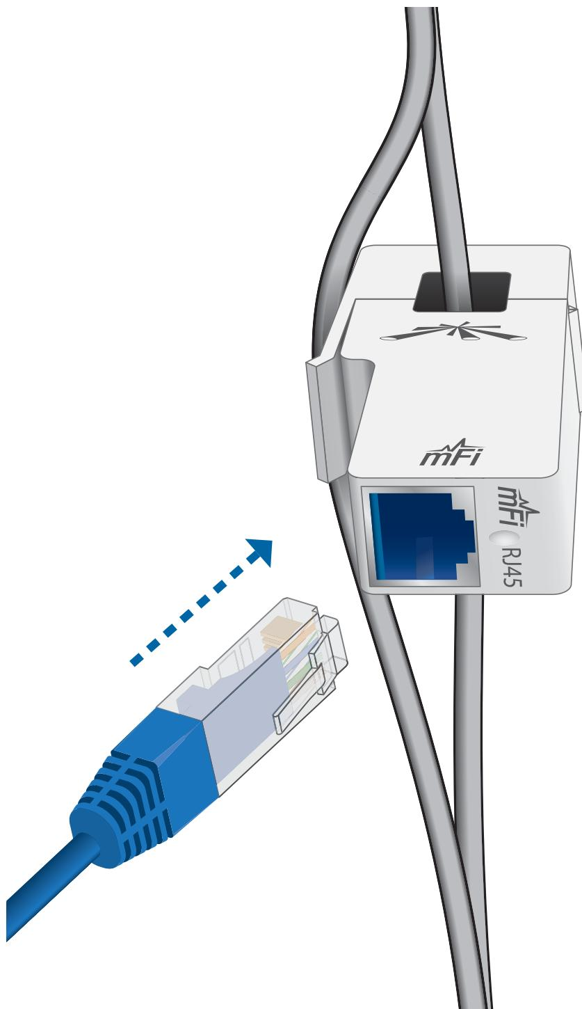
5. Connect the other end of the CAT5/6 cable from the mFi Current Sensor to an mFi RJ45 port on the mFi mPort.
