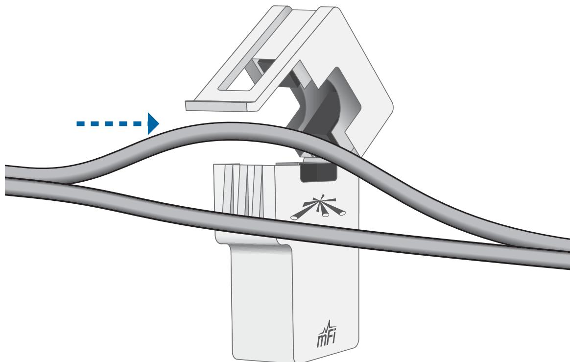
**3. Close the opening of the mFi Current Sensor until the latch snaps into place.**
