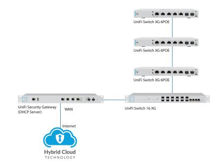
Multiple switches are daisy-chained through their SFP+ interfaces.
