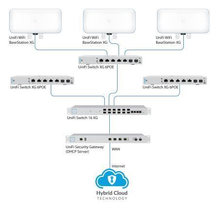
Multiple switches connect via SFP+ to the UniFi Switch 16 XG. One UniFi Switch XG 6POE delivers data and 802.3bt PoE++ to multiple APs, the UniFi BaseStation XG, model UWB-XG.
