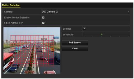
Figure 8-2 Set Detection Area and Sensitivity
