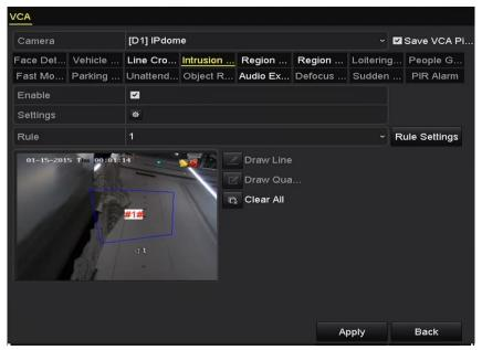
Figure 10-9 Draw Area for Intrusion Detection
