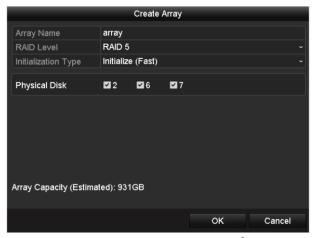
Figure 13-8 Create Array Interface
