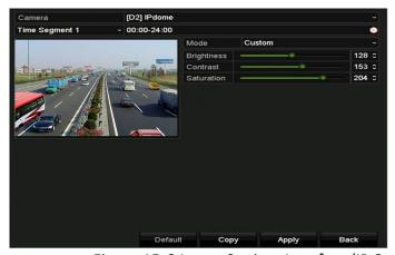
Figure 15-6 Image Settings Interface (IP Camera)
