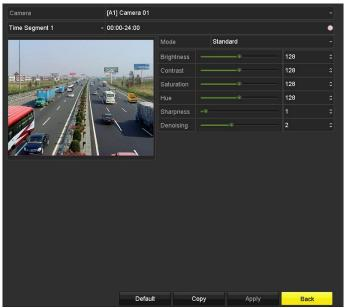
Figure 15-5 Image Settings Interface (Analog Camera)
