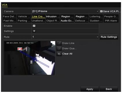
Figure 10-7 Draw Line for Line Crossing Detection
