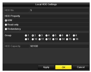
Figure 14-13 Local HDD Settings Interface
