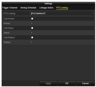
Figure 8-9 Set PTZ Linking of Alarm Input
