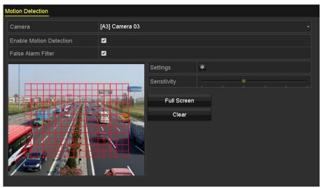
Figure 5-16 Motion Detection- Mask
