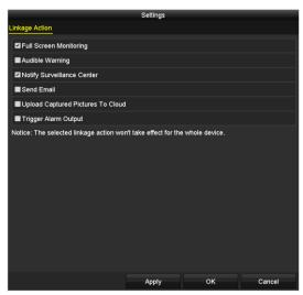
Figure 8-11 Disarm Linkage Actions
