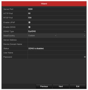
Figure 2-24 Set Advanced Network Parameters
