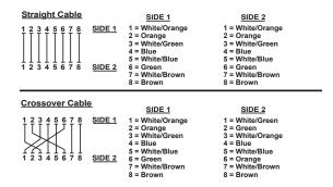
Figure B-1: Straight-through and Crossover Cables
