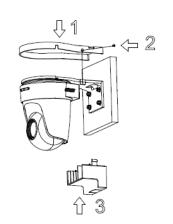
D. Install other parts of the bracket in sequence
