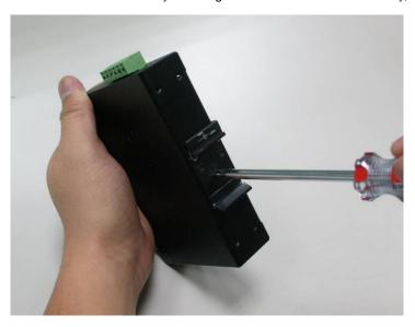
Step 1: Screw the DIN-rail bracket on the Industrial Cellular Gateway.
