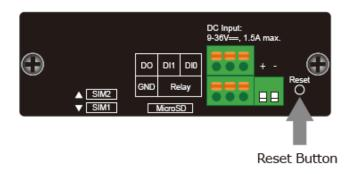
Figure 2-3 Rest Button of ICG-2510W(G)-LTE Series
