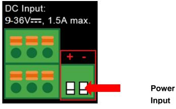
Figure 2-5: Wiring the Power Inputs
