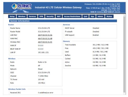
Figure 3-2 Web Main Screen of Industrial Cellular Gateway
