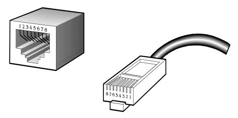
The standard RJ45 receptacle/connector
