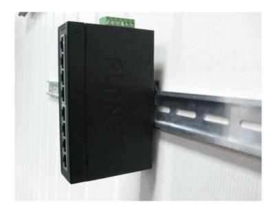
**Step 3:** Check whether the DIN-rail bracket is tightly on the track.
