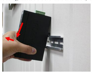
Step 5: Lightly pull out the bottom of DIN-rail bracket to remove it from the track.
