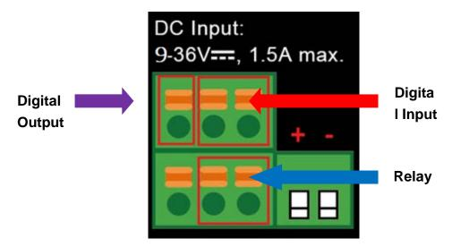
Figure 2-6 Wiring the DI/DO Inputs and Relay
