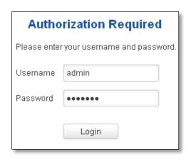
Enter the default password, which is "admin01" into the "Password" field and then either click Login with your mouse or press the Enter key. You have now successfully logged into the RUT850!
