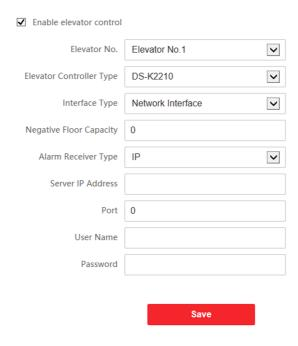
Figure 5-22 Elevator Control
