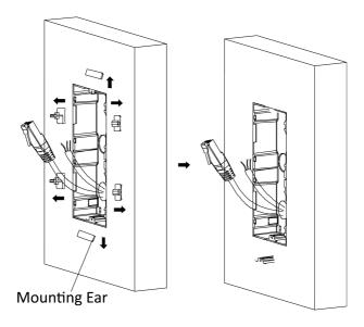
Figure 3-26 Remove the Mounting Ears
