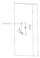
Figure 3-16 Drill Screw Holes
