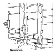
Figure 3-56 Remove the Plastic Sheets
