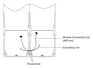
Figure 3-46 Place the Grounding Line and Module-Connecting Line
