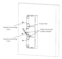
Figure 3-33 Placement of Lines
