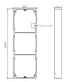
Figure 3-29 Mounting Frame
