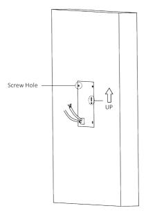
Figure 3-3 Drill Screw Holes
