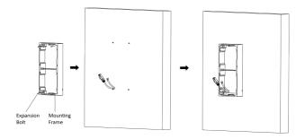
Figure 3-17 Fix the Mounting Frame
