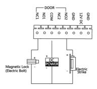
Figure 2-5 Door Lock Wiring
