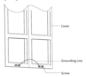
Figure 3-51 Connect the Grounding Line to the Cover
