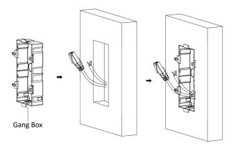
Figure 3-24 Mark the Screw Holes
