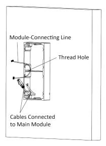
Figure 3-18 Placement of Lines
