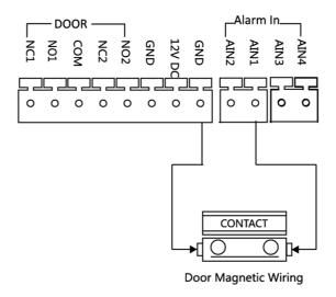
Figure 2-6 Door Contact Wiring
