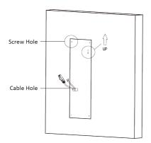
Figure 3-30 Drill Screw Holes
