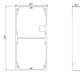
Figure 3-15 Mounting Frame
