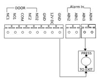
Figure 2-7 Exit Button Wiring
