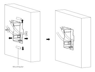
Figure 3-12 Remove the Mounting Ears
