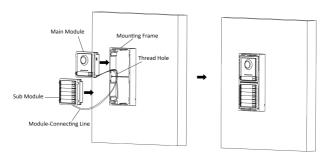
Figure 3-20 Insert the Modules
