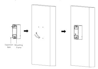
Figure 3-4 Fix the Mounting Frame
