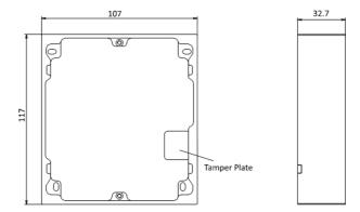
Figure 3-2 Mounting Frame
