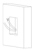
Figure 3-23 Drill the Installation Hole
