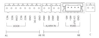
Figure 2-2 Two-Wire Main Unit Terminal
