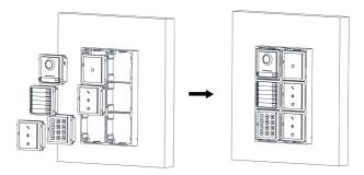
Figure 3-50 Insert the Modules
