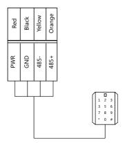
Figure 2-8 RS-485 Card Reader Wiring
