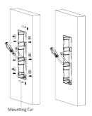
Figure 3-41 Remove the Mounting Ears
