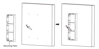
Figure 3-31 Fix the Mounting Frame
