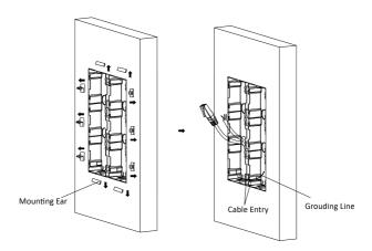
Figure 3-59 Remove the Mounting Ears
