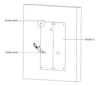
Figure 3-45 Drill Screw Holes
