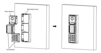
Figure 3-35 Insert the Modules into the Frame
