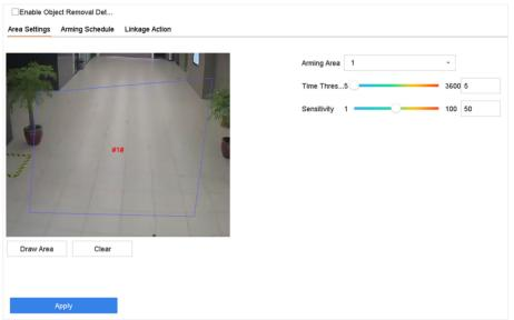
**Figure 5-9 Object Removal Detection**
