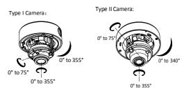
Figure 2. 4 3-Axis Adjustment
