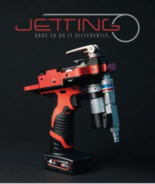
Robust handheld battery powered fiber blowing tool optimized for FTTX installation of blown fiber (EPFU) and micro/nano cables, from 0,8 to 3 mm into duct size 3, 5 and 7 mm. The effective fiber security, and adjustable clamping force secures that all cable designs can be installed effective and safe. Delivered in strong transport case with batteries, charger and an assortment of cable seals. Ready to blow!
