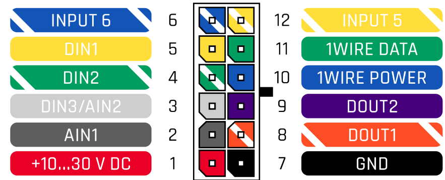
Figure 2 FMB122 2x6 socket pinout
