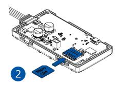
Figure 5 Micro SIM card insert
