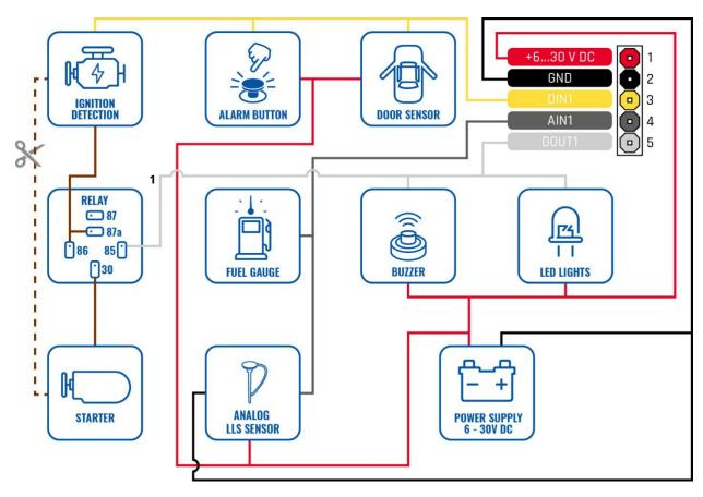
Figure 3 MTB100 Wiring scheme
