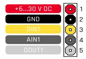
Figure 2 MTB100 pinout
