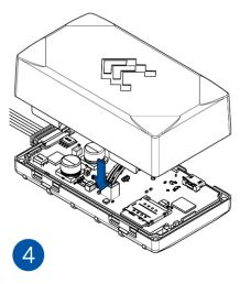
**Figure 7 Attaching cover back**
