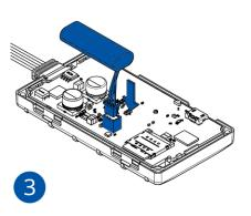
**Figure 6 Battery connection**
