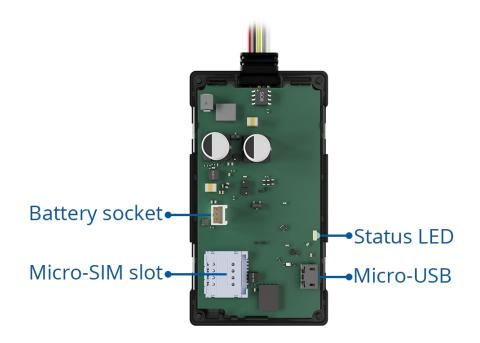
Figure 1 MTB100 device view
