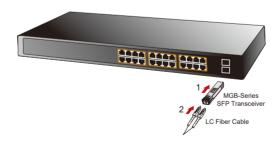
Figure 5-3: Plug In the SFP Transceiver
