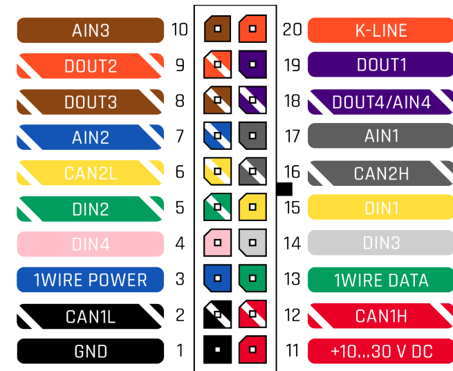
Figure 2 FMB640 Pinout
